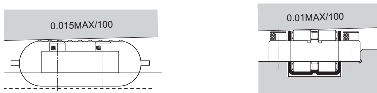
(a) Parallelism between the LM Roller and the raceway (b) Allowable tilt of the roller in the longitudinal direction
