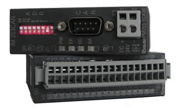
Each CANopen bus coupler handles up to 8 modules. The individual module can interface digital or analogue signals. The assembly is extremely simple. The RIO system modules are snapped on the bus connector which is securely fastened on a 35 mm standard rail.
